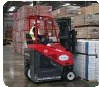
*Timbmet's CBs stack packs of flooring from the ground up for space saving in the warehouse*
