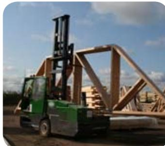
Pinewood Structure's 5t SL handles 12m lengths of engineered wood, heavy packs of timber and bulky roof trusses
