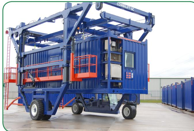
The SC has a 35t capacity and offers complete independence for the transportation of containers and similarly oversized loads. It benefits from a much lower axle weight than reach stackers or container handling forklifts and is therefore ideally suited for
